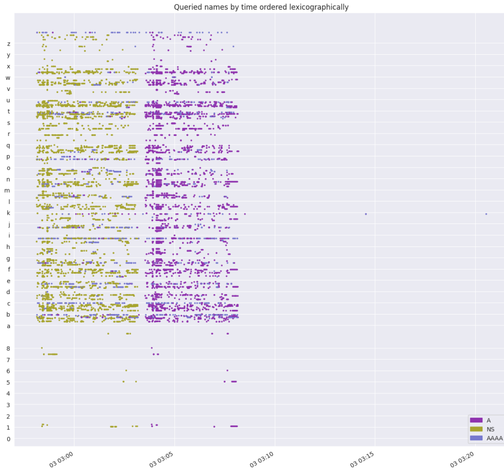
Figure 4.13: A scanning operation asking for NS records first, then for A records in a second phase (time frame = about 25 minutes)
